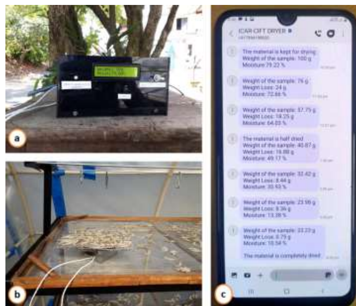
Fig 2. Mobile alert system for shrimp drying in a solar tunnel dryer
